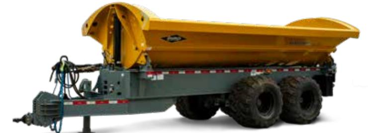
20-to 30-ton capacities ◀ Off-road construction and Ag ▶ Construction grade or flotation tires ▶ Can pull in train
