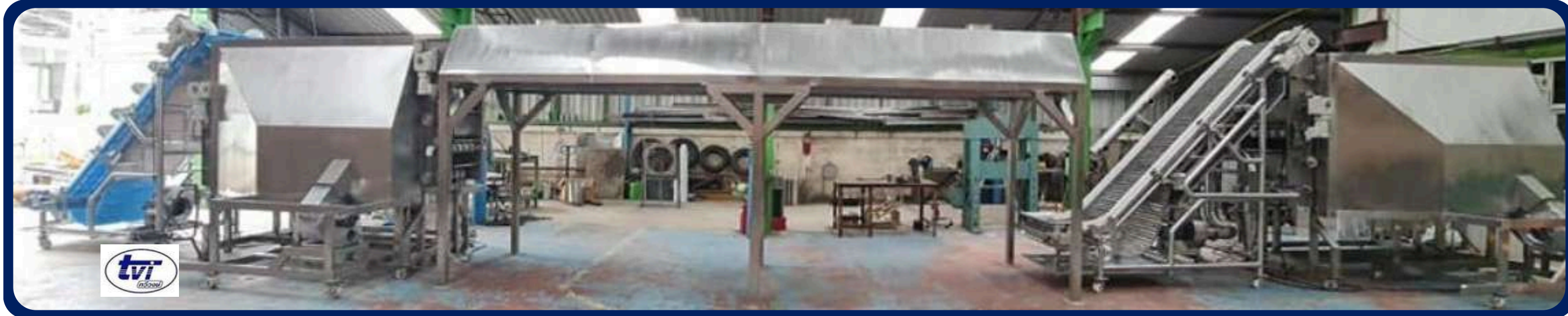
Air cooling and de-oiling conveyor system
