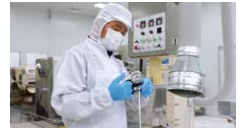
8. Checking for Proper Thickness.
