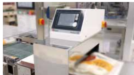
10. Inspecting Packaged Noodles with Metal Detectors.
