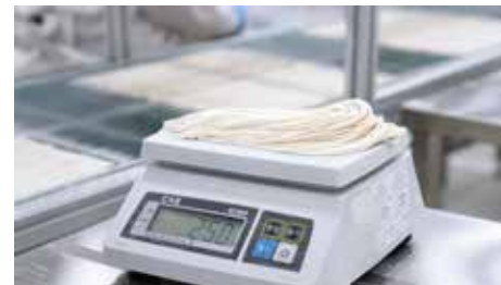
7. Ensuring Consistent Weight by Checking Yarn Weight.
