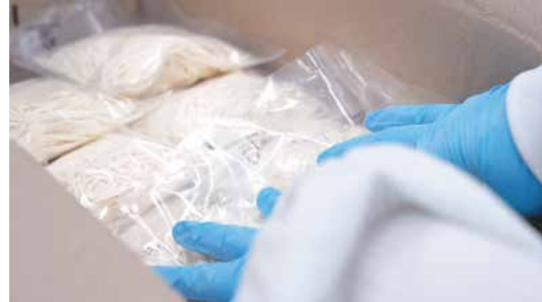
4. After inspection with metal detectors and weight sorters, the packaged noodles are placed into boxes for packaging.
