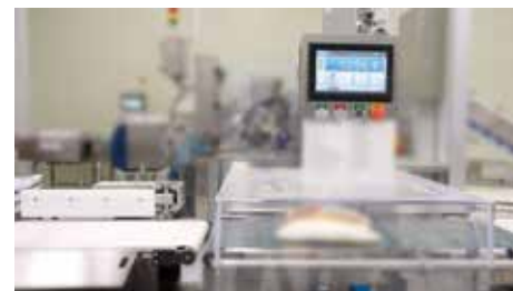
11. Inspecting Packaged Noodles with Weight Sorters.
