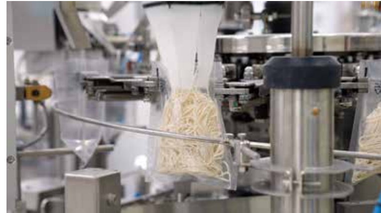
2. The noodles are automatically packaged into packaging paper.
