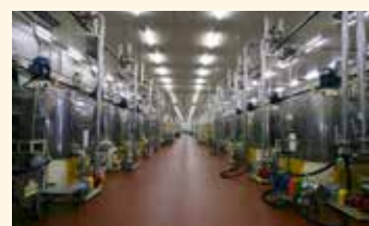
04 Conching facilities Evaporation of moisture, deodorizing, viscosity and scent control
