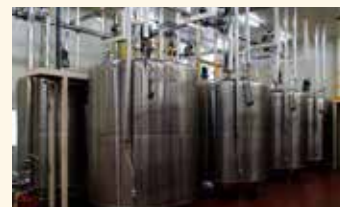
05 Tempering facilities Stabilization of crystals, maintaining deep flavor and gloss, creating smooth texture
