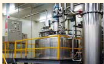
09 Concentrating Facilities : Concentrate water-based beverages, smoothies, liquid tea, etc
