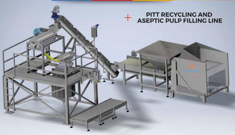
Prunext International developed a technology to recover pits and pulp from the pitting process for use as fuel in boilers with biomass burners. The recovered pulp is pasteurized and aseptically packaged in bags before being sold. All of this is the result of our ongoing dedication to innovation and the optimization of all of our clients' manufacturing processes.
