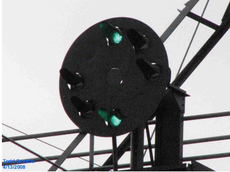
Amtrak PCL's at the south end of the Halethorpe MARC station (SW suburban Baltimore), and a pair in Wilmington with LED's.
