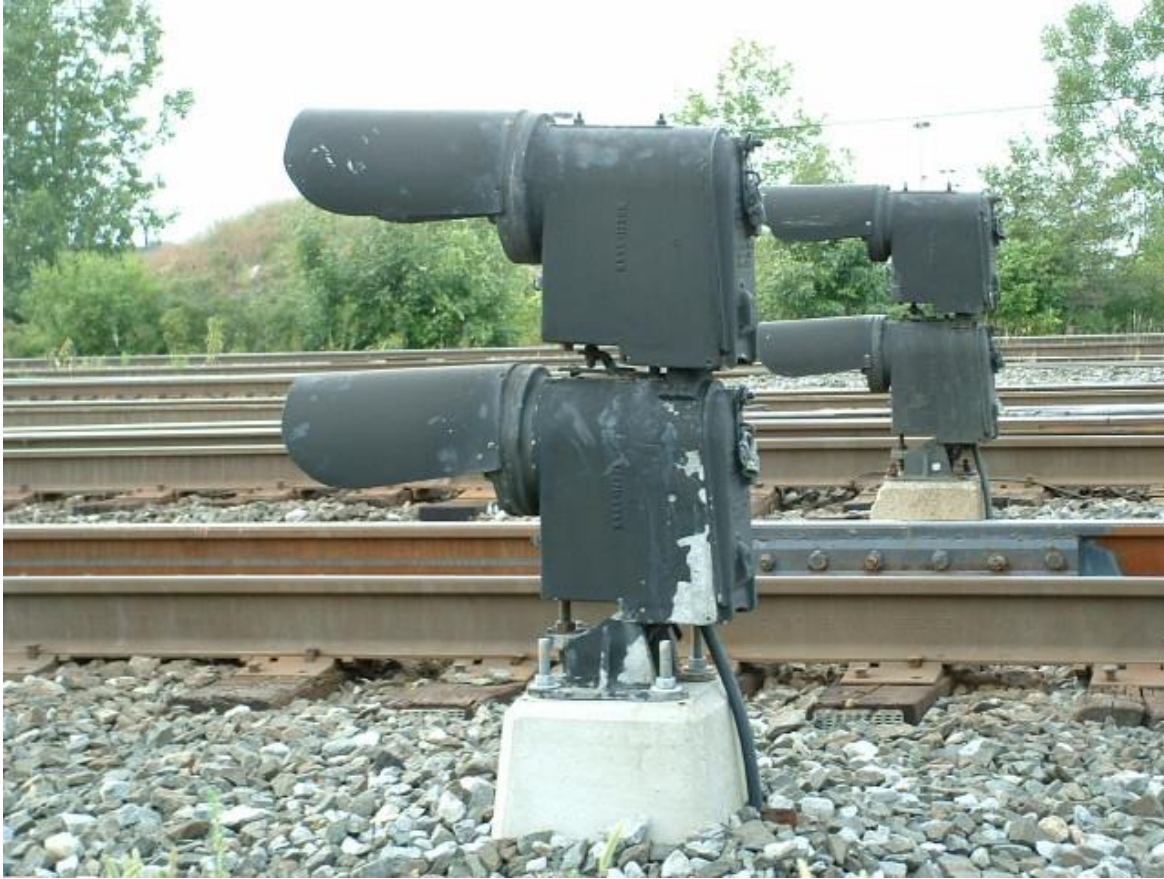
A couple of dwarf searchlight signals in Buffalo NY, on the former New York Central (now CSX). These are GRS units, the giveaway being the hoods - notice the difference in their shape from the US&S hoods above.
