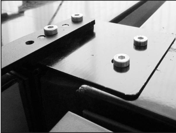
3. Place the top plate over the screw holes and remount hinge screws and add the 2 extra screws in the other cabinet
