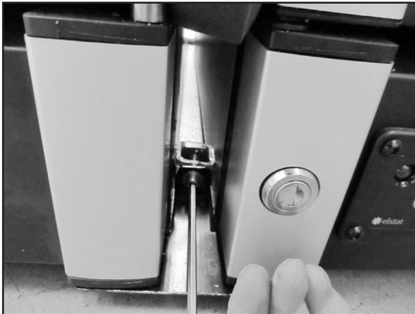
5. Tighten the screw, so the rubber hose bush against the cabinets. Replace the Rubber sealing
