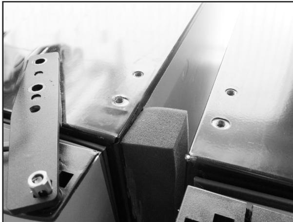
2. Remove the bolts that holds the top hinge.
