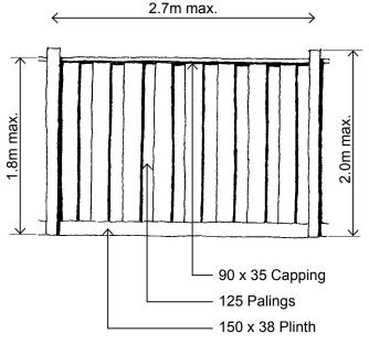
Diagram 10 - Corner Fence Elevation
