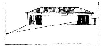
Diagram 6 - Excessive earthworks approach to topography
