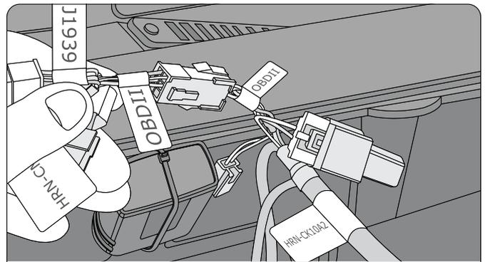
**Step 6B:** Connect the OBD II-labelled 6-pin white Molex connector from the HRN-CK10A2 harness to the OBD II-labelled 6-pin white Molex connector from the HRN-CM24Y1 harness.
