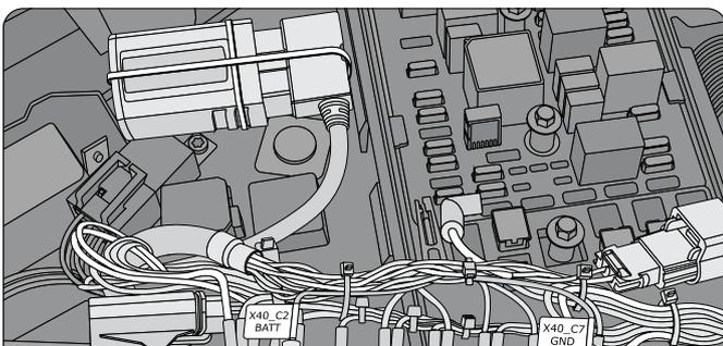
**Step 7:** Plug in the GO device, and use zip ties to secure the device and harnesses.
