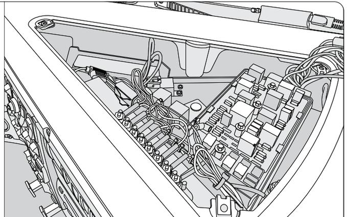
**Step 2 :** Connect the red wire from the HRN-CK10A2 harness (labeled **BATT**) into the second pin (labeled **Battery** on the bus bar).
