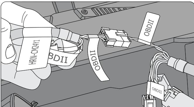
**Step 6A :** Connect the OBD II-labelled 12-pin black Molex connector from the HRN-CK10A2 harness to the OBD II-labelled 12-pin black Molex connector from the HRN-CM24Y1 harness.
