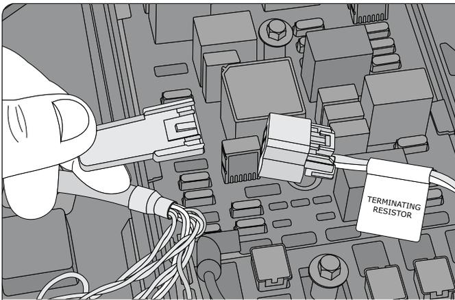
**Step 4B:** Locate the 2-pin J1939 connector in the fuse box and remove the EOL resistor.
