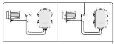
**2.** To add any additional IOX accessories, remove the Termination Shunt. Use the zip ties provided to secure the connection.
