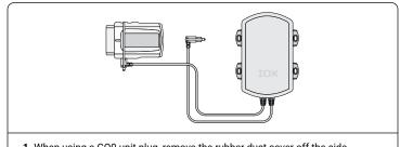
**1.** When using a GO9 unit plug, remove the rubber dust cover off the side of the GO9 and plug in the IOX-BATTERY. Use the zip provided to secure the connection.
