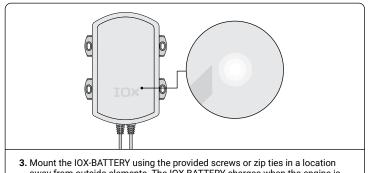
Mount the IOX-BATTERY using the provided screws or zip ties in a location away from outside elements. The IOX-BATTERY charges when the engine is running. The blue LED light illuminates when charging.
