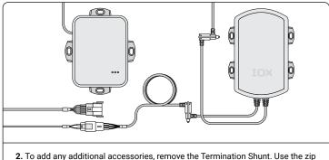
To add any additional accessories, remove the Termination Shunt. Use the zij ties provided to secure the connection.
