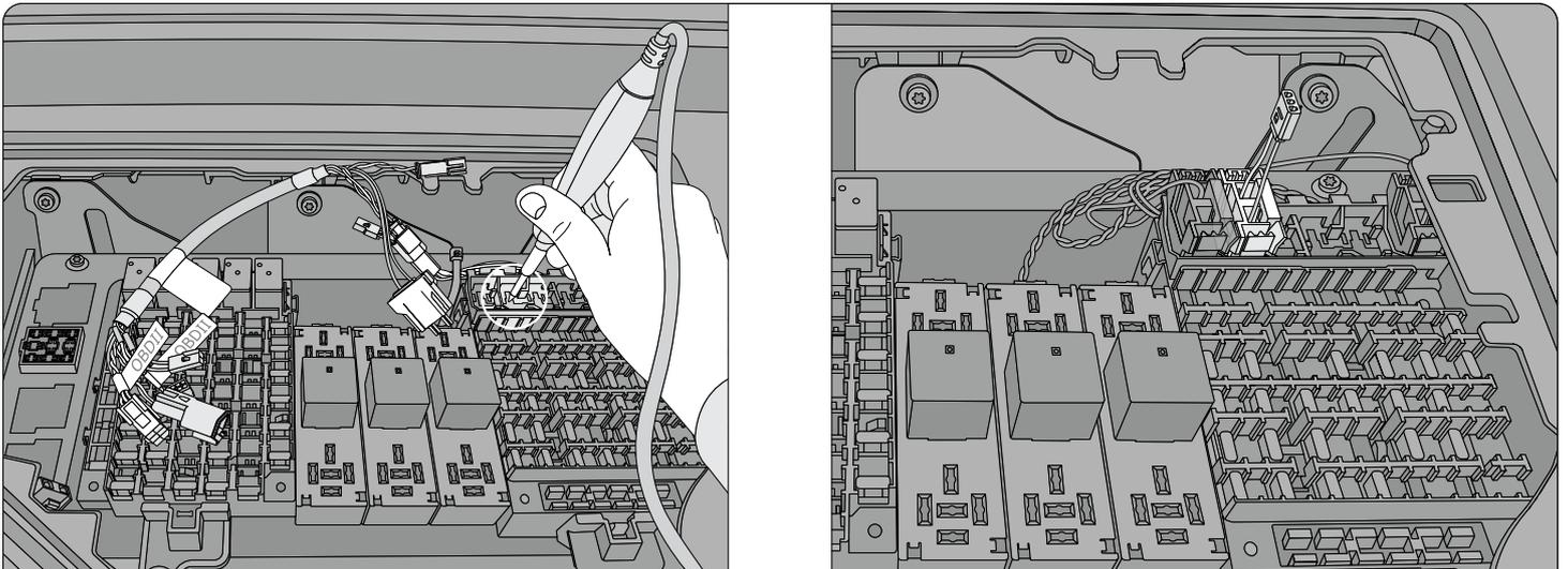
**Step 2:** Connect the 2-pin white connector from the kit into any spare constant power slot. Test for power with a multimeter to verify.
