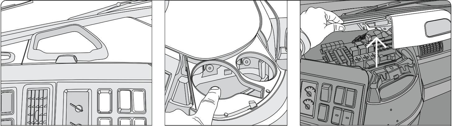
**Step 1:** Remove the two T-25 screws holding the fuse box cover in place, then pull gently upward to remove the cover.
