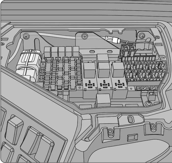
**Note:** Connect the HRN-CM24Y1 to the GO device. Secure the GO device to the harness using a zip tie. Secure the GO device to the frame of the fuse box using two additional zip ties.
