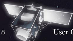
Artist view of the NAOMI design, with focal plane projection on Earth; here 3 retinas are implemented to cover the swath.
