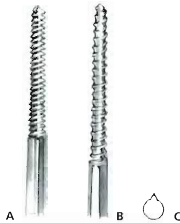
FIGURE 4-108. The Orthofix screws differ from the Schantz screws used on the Wagner device and others in their thread design: they are tapered. This is thought to give them a more secure fit in the bone. The standard cortical screw ( A ) tapers from 6 mm at the base of the thread to 5 mm at the tip (6/5 mm). Smaller screws of 4.5/3.5 mm are also available (to be used in bones with a diaphyseal diameter less than 15 mm), as are 6/5 mm cancellous screws ( B ). For leg lengthening, these screws are available with a cutting edge ( C ) to minimize the tissue trauma at the leading edge of the screw during lengthening.
