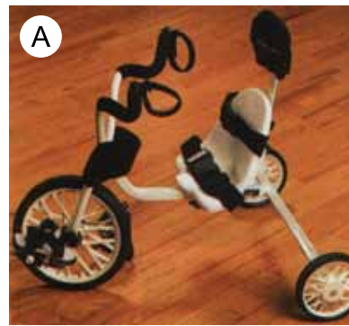
Special tricycle with modified handles, head rest and restraints for the body.
