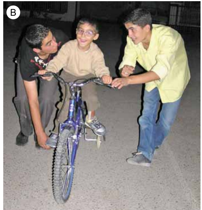
Two small rear-wheels are added to a standard bicycle for better balance.
