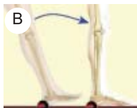
Heel (first) rocker: The period from the moment the heel strikes the ground to the moment the forefoot touches the ground. The pivot of motion is the heel.
