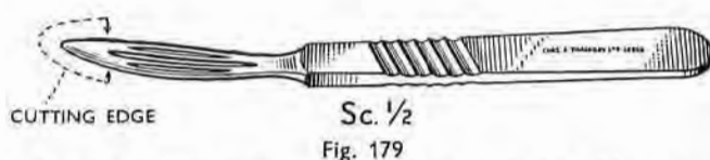
Knife for dividing moorings of talus from within the ankle joint. (It is a Kocher's dissector toughened and sharpened.)
