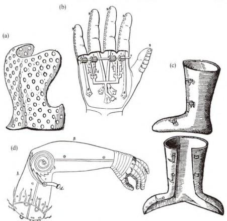
Figure 107 Paré: various devices (a) scoliosis corset; (b) wrist and hand prosthesis; (c) club-foot boot; (d) artificial arm
