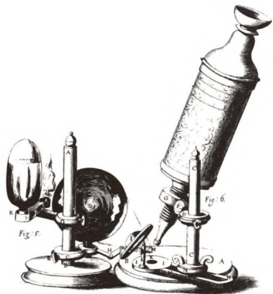
Microscope used by Robert Hooke, and Hooke's drawing of a flea. From Hooke's book 'Micrographia', 1665. Hooke worked for the Royal Society of London, founded in 1662 to encourage scientific knowledge.
