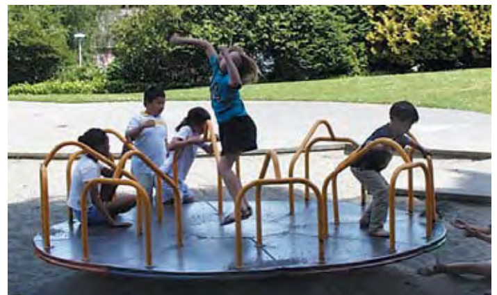
Fig. 11.62 Playground equipment. Reduce risk by providing soft surfaces (sand) and playground equipment of limited height to reduce fall distance.
