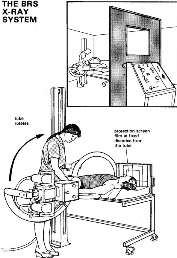
**Fig. 1-8 THE BRS X-RAY SYSTEM** was developed by WHO to make essential cost-effective radiology available safely and reliably all over the world. If you want one of these machines, order one made to WHO specifications. Note the screen protecting the operator.
