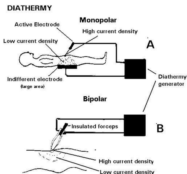
**Fig. 3-5 DIATHERMY.** A, monopolar diathermy produces high current density at the active electrode dissipated through the body tissues through the 'indifferent' electrode with resulting low current density. B, bipolar diathermy produces high current density across insulated diathermy forceps tips. After Sear JW, Rosewarne F. *Anaesthesia for Surgeons, Oxford Textbook of Surgery, OUP 1994 p.83 Fig.2,3.*
