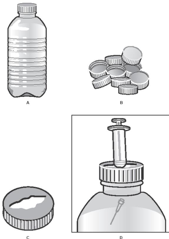
**Fig. 5-2 LOW-COST SHARPS CONTAINER WITH NEEDLE REMOVAL DEVICE.**
