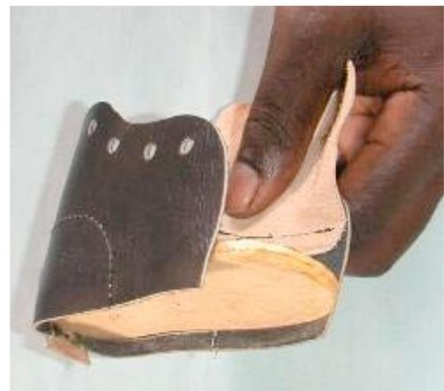
Apply glue on the outside edge of the outersole and on the leather that was left over as lasting allowance. Let it dry and connect both parts by folding the leather onto the plywood. Hammer gently to get good bonding (see fig. 36 & 37).
