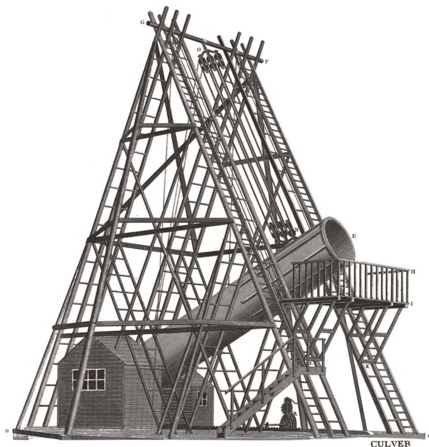
Sir William Herschel's 40-foot telescope built in 1789; he studied planet rotation, catalogued over 800 double stars; in 1781 he discovered the planet Uranus.
