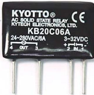
NOTE: These particular relays have a very low leakage current, so these aren't necessarily ideal for running powerheads. I however use them in my build, and they work great with the Hydor Koralia Powerheads. I went with SSR's because they are completely silent. You can easily substitute mechanical relays with similar specs. They are much less expensive, but make noticeable clicking sounds when activated.
