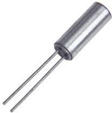
NOTE: This is the clock source for the RTC chip
