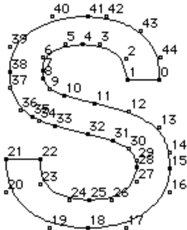
Figure 1-2 A glyph description consisting of a series of on and off curve points
