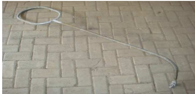
Gambar 32 Arcing horn sisi tower
