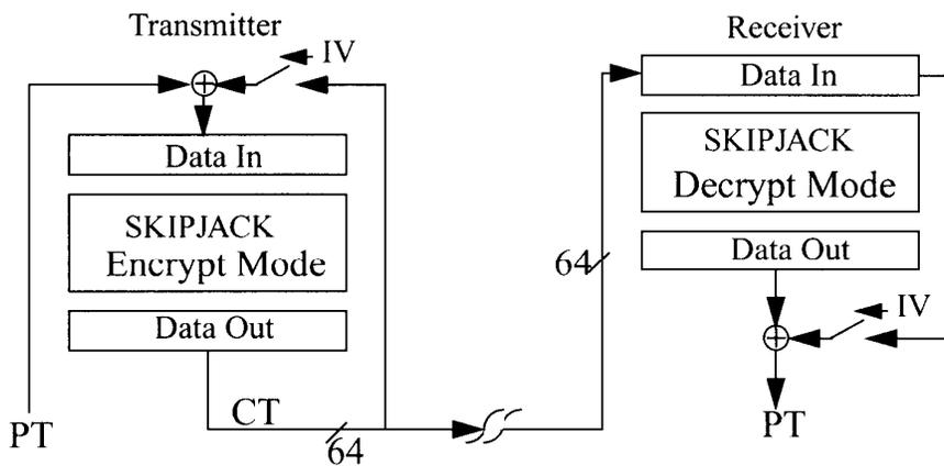
Figure 4. "Cipher-Block Chaining Mode Diagram"
