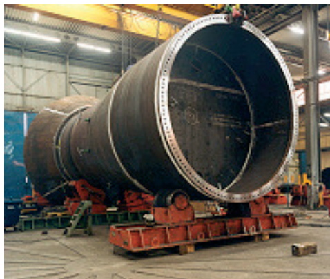
Figure 5.2 Wind turbine monopile foundation at Sif factory
