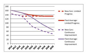
When emissions levels are being reduced, the fleet average emissions in a given year will always lag behind those of new cars from that year. For example, if 10% of the car fleet is replaced with new cars which are 10g/km better than the fleet average, they will only improve the fleet average by about 1 g/km overall. If the average emissions of new cars entering the fleet levelled off and remained constant over some years, then the fleet
