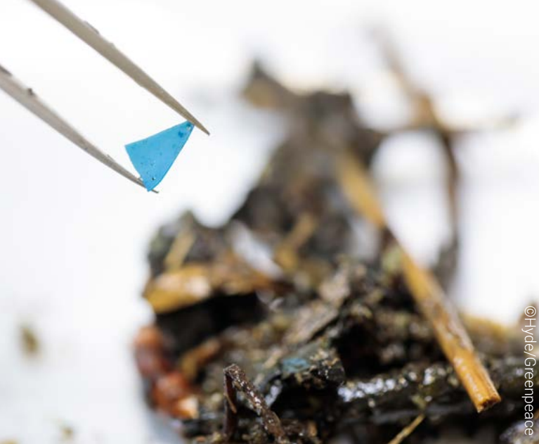
Plastic sample from the River Mersey, showing a microplastic particle being separated from organic material at Greenpeace Research Laboratories, 17 Apr 2019.
