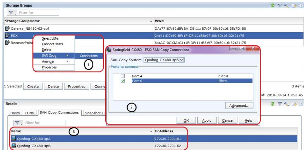
**Figure 35: LUN masking procedure**
