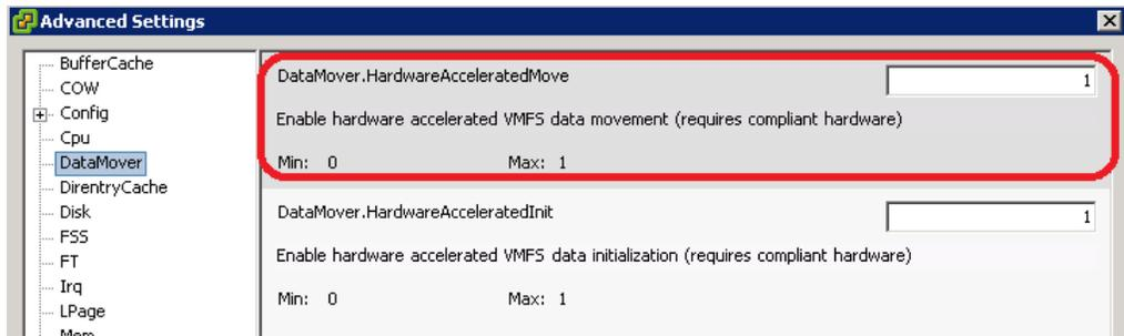
**Figure 9: Hardware acceleration settings**
