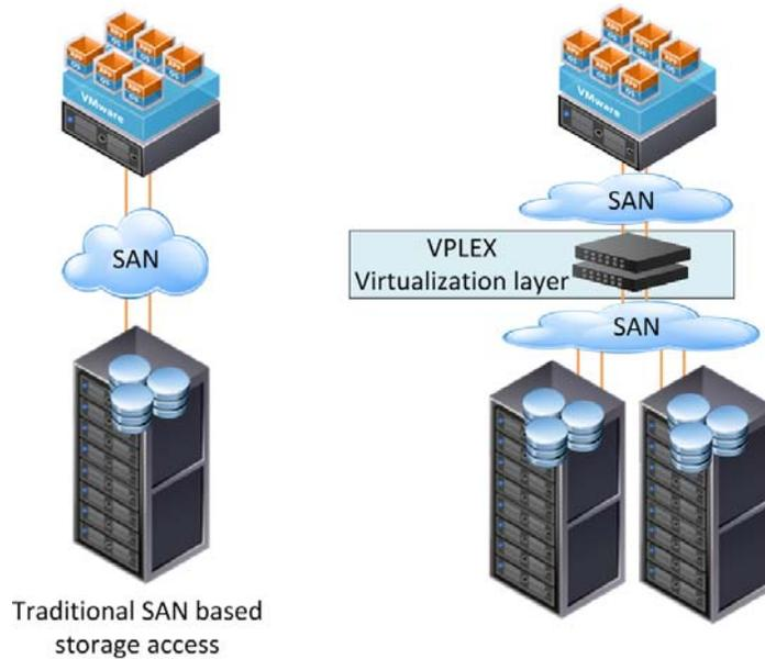
**Figure 23: Architectural differences between SAN-based and VPLEX storage**
