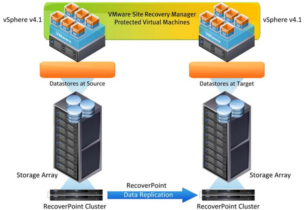
**Figure 53: Test environment for VMware vCenter Site Recovery Manager**
