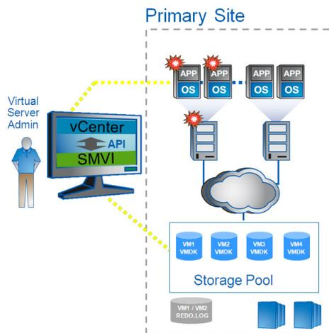
Figure 3) Virtual infrastructure and associated storage during an SMVI backup
