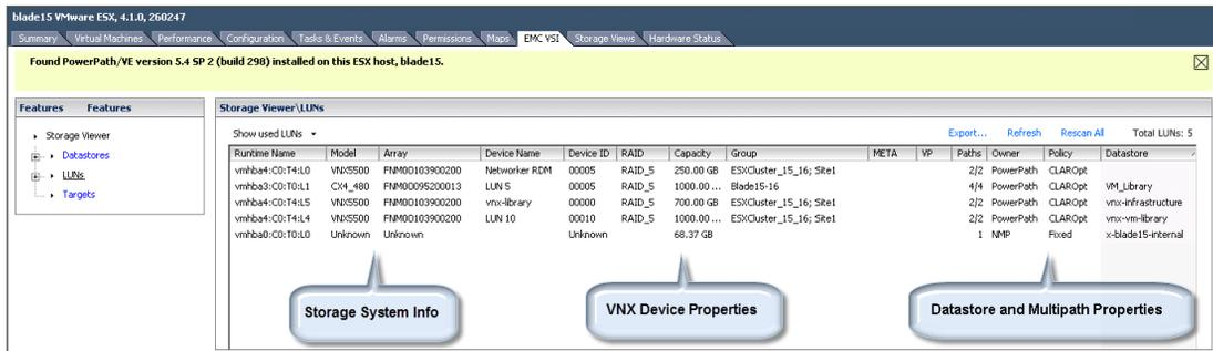
Figure 6 Storage Viewer VNX block storage details
