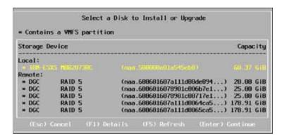
To confirm the correct boot disk, press **F1** to display details about the disk. After viewing the disk details, press **Enter** to close the pop-up.
