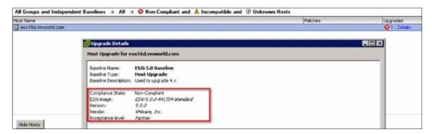
If a host returns a status of **Incompatible** with the reason being an invalid boot disk, you cannot use Update Manager to upgrade. Try using the ESXi Installer.
