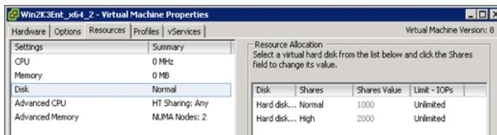
Next, we will modify the iometer settings. We will set the value for outstanding I/O to be **64**. This should mean that the latency value for I/Os becomes high enough (greater than 30ms) to trigger congestion. This should also mean that SIOC will consider the virtual machine with 1000 shares to have a lower priority than the virtual machine with 2000 shares regarding the scheduling of I/O.
