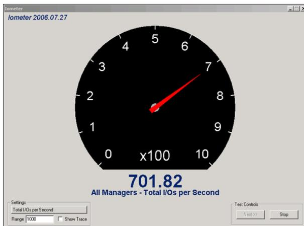
Repeat these steps using the same configuration setup (4K I/Os, 75% Read, 0% Random) on the other virtual machine on the other ESXi server. Leave Iometer running on both virtual machines. I/O is now being generated to the same shared datastore from two virtual machines on two different ESXi hosts.
