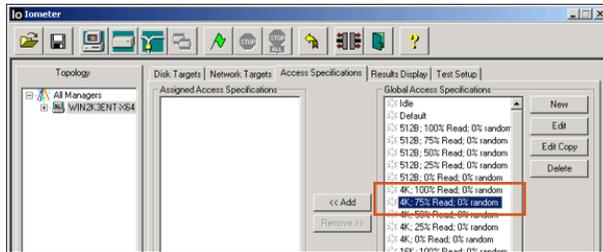
Finally, select the **Results Display** tab. You should see that the **Update Frequency** is set to 2 seconds. Click the **green flag icon** to start the I/O. Save the results file to the default location. In the **Results Display** tab, you can now begin to see IOPS and latency information being updated every 2 seconds.
