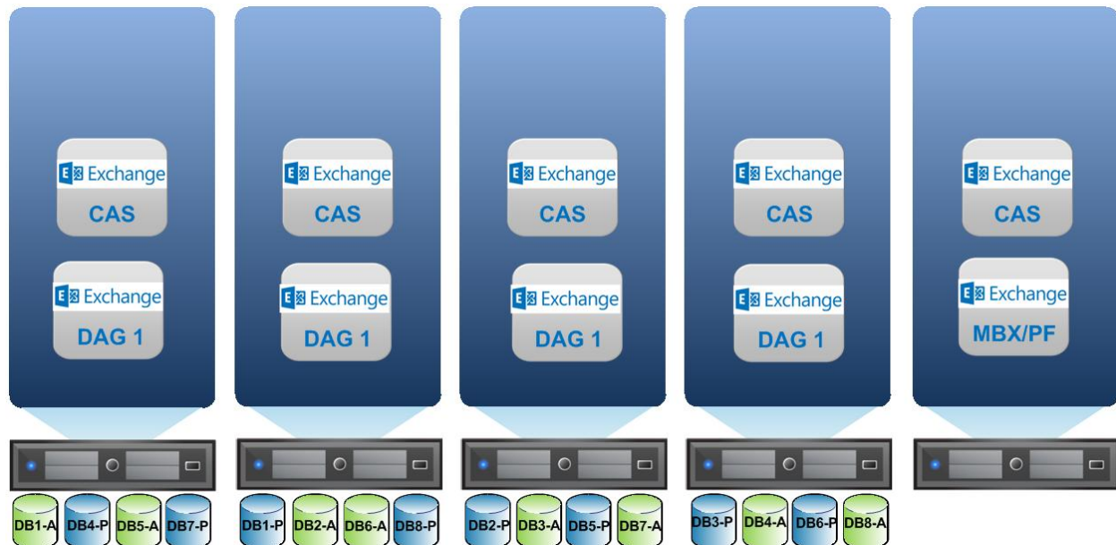
Figure 3. Normal State Exchange 2013 DAG with vSphere HA
