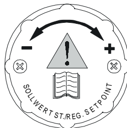
Figure 8: Spring Pressure Regulator Adjustment Knob
