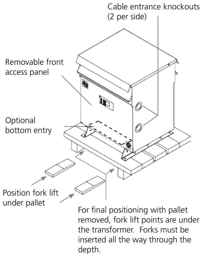
1. Handling - units are designed to be raised by a fork lift from underneath the pallet. Final positioning of the unit with the pallet removed can be via a fork lift under the transformer with the forks between the channels.
