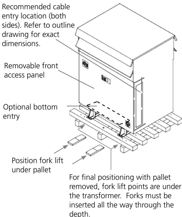
1. Handling - units are designed to be raised by a fork lift from underneath the pallet. Final positioning of the unit with the pallet removed can be via a fork lift under the transformer with the forks between the channels. **(Note: Transformers weighing greater than 2350 lbs should be lifted by removing the top panel and accessing the lifting provisions on top of the top of the core and coil.)**
