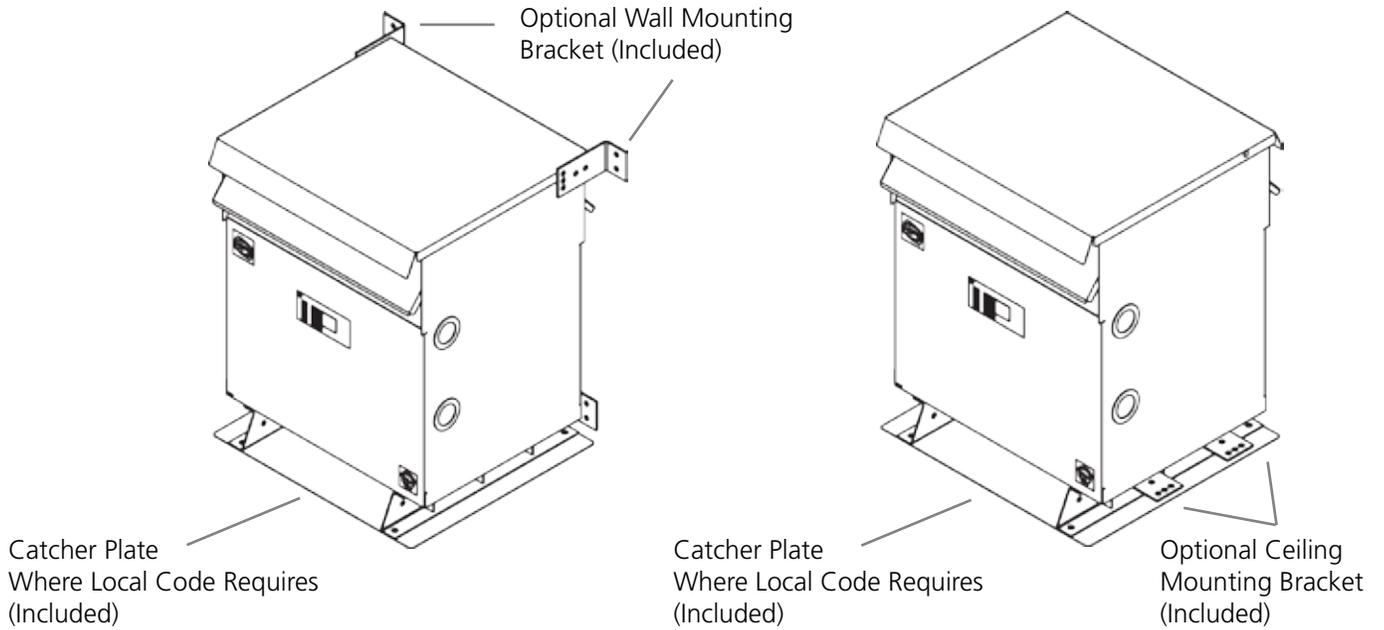
LOCATION OF WALL MOUNTING BRACKETS AND CATCHER PLATES FOR TYPE 3R ENCLOSURES
