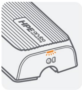
Figure 16. HPE Aruba Networking User Experience Insight Sensor showing LED position
