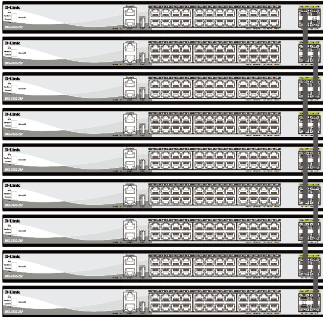
Figure 0-3 Duplex Chain stacking topology (SFP28 ports)
