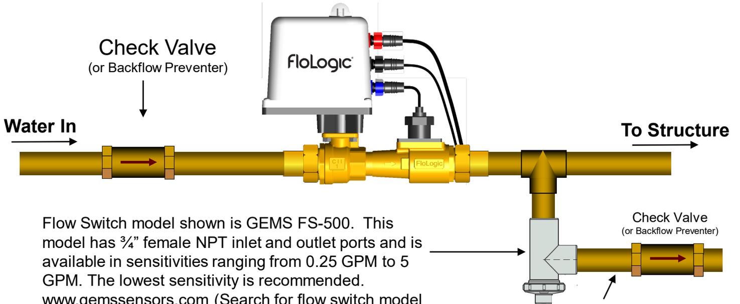
Flow Switch model shown is GEMS FS-500. This model has 3/4" female NPT inlet and outlet ports and is available in sensitivities ranging from 0.25 GPM to 5 GPM. The lowest sensitivity is recommended. [www.gemssensors.com](http://www.gemssensors.com) (Search for flow switch model number based on pipe size)
