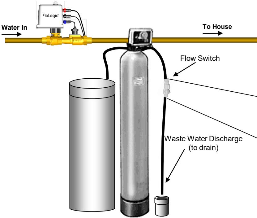
**NOTE:** Flow switch is installed on the discharge line. Switch state is Normally Open and closes when flow is detected. Switch shown is from GEMS Sensors at [www.gemssensors.com](http://www.gemssensors.com). (search for flow switch model based on discharge rate and pipe size) Also available through other retailers.
