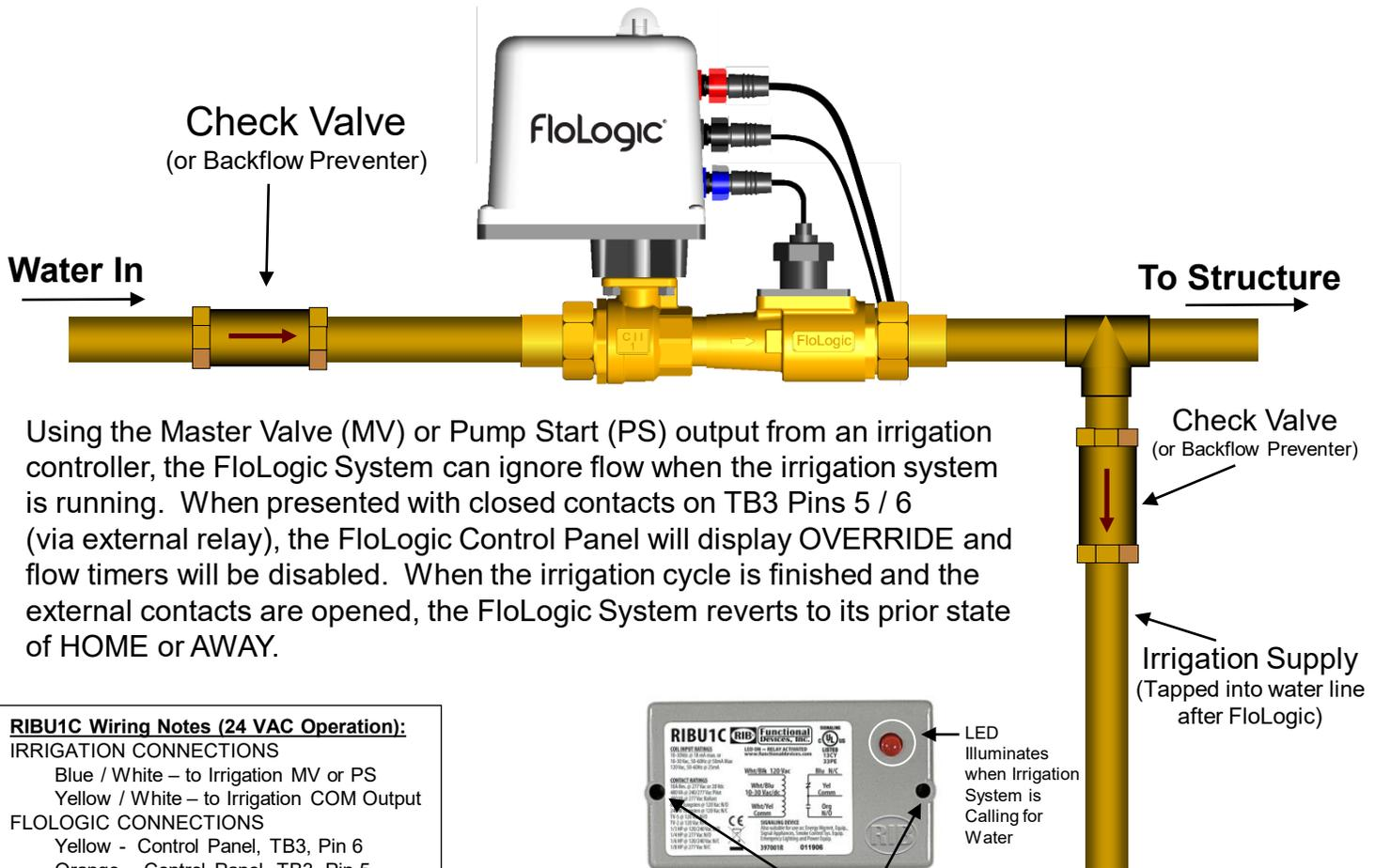
Using the Master Valve (MV) or Pump Start (PS) output from an irrigation controller, the FloLogic System can ignore flow when the irrigation system is running. When presented with closed contacts on TB3 Pins 5 / 6 (via external relay), the FloLogic Control Panel will display **VERRIDE** and flow timers will be disabled. When the irrigation cycle is finished and the external contacts are opened, the FloLogic System reverts to its prior state of HOME or AWAY.
