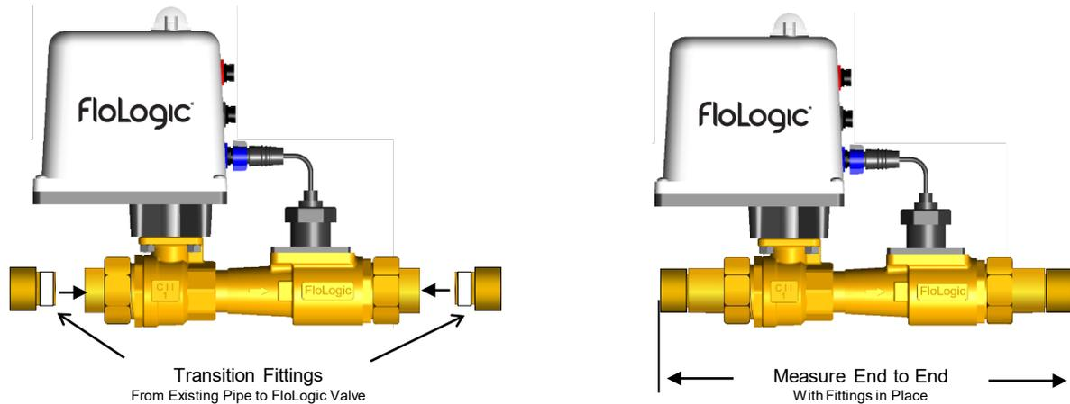
Carefully measure the overall length of the assembled Valve and fittings. Take this measurement and mark it on the water pipe where you intend to locate the FloLogic Valve. Next, determine how far the pipe will insert into each of the transition fittings when assembled after cutting. Reduce the width of the overall measurement by these insertion lengths. Mark the reduced overall length on the pipe and prepare to cut the pipe.
