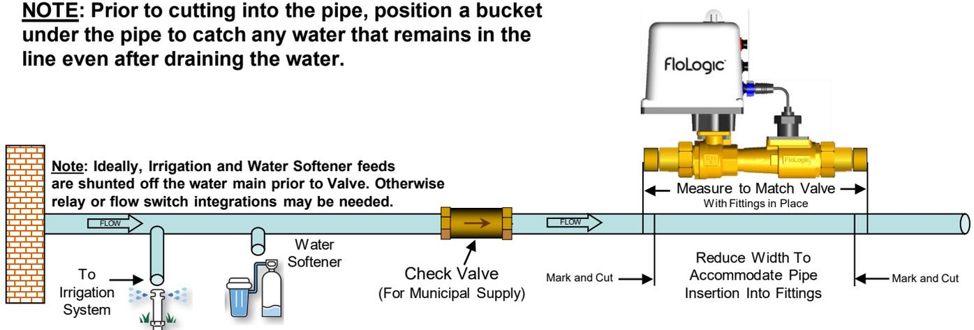
Using the appropriate tools, cut the pipe in the places marked. Be careful to make a clean, square cut to ensure minimal clean-up and prep work before installing the fittings. Additional pipe supports may be required if the cut pipe sags excessively.
