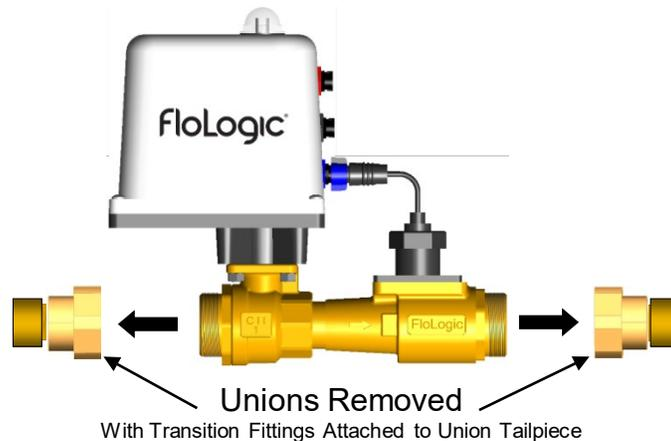
Dry fit the transition fittings onto the water line you cut in Step 5. If there is enough clearance for the union nut to slide over the transition fittings and onto the pipe, slip the union nut down the pipe and out of the area where you will be attaching the fittings to the pipe.
