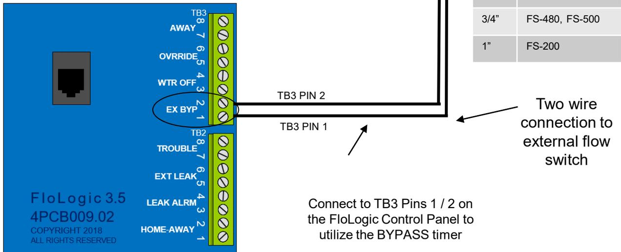
When connected to EX BYP input, the bypass timer will be started when water flow is detected in the discharge tube and the display will read EX.BYPASS alternating with HOME or AWAY.
