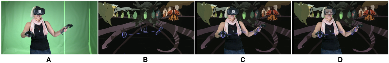
Figure 1: Mixed Reality Overview: VR user captured in front of green-screen (A), blended with her virtual environment (from Google Tilt Brush ) (B), to generate the MR output: Traditional MR output (C) has the user face occluded, while our result (D) reveals the face. The headset is deliberately rendered translucent instead of being completely removed.
