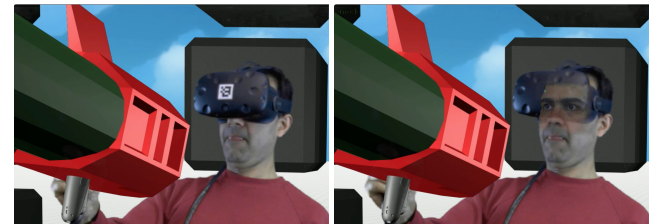
Figure 3: Before (left) and after (right) headset removal. Left image also shows the marker used for tracking.
