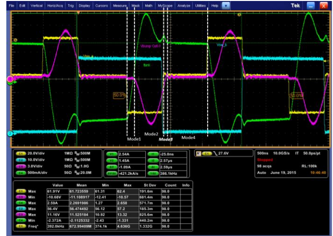
Figure 32 Experimental results: CH1-Yellow: V_p ; CH2-Blue: V_{ds} of FET D; CH3-Pink: V_{p\_sec} ; CH4-Green: -i_{res\_prim} ; i_{res\_prim} peak=2.54A, reflected i_{res\_sec} peak=17.8A, i_{park} =10.5A, f_{sw} =386kHz, I_o =25A
