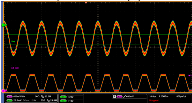
Figure 40 Load transient performance at 100kHz switching, 0-25A, 12.5A/ \mu s (CH3-Pink: current reporting signal for the load tester, 15mV/A; CH4-Green: Output Voltage with 20MHz BW)
