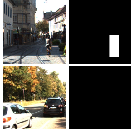
Fig. 5. Examples of a stop (top) and go (bottom) instances and the corresponding proxy labels (right). The proxy label contains the full bounding box over pedestrians and bicyclists as a binary mask.
