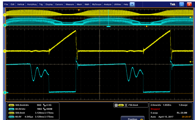
Figure 28 Final Waveform with the solution A and B implemented, 120Vac input, 20W output
