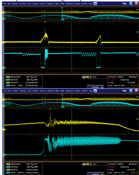
Figure 27 Experimental results of the ringing in cascode structure, 120Vac input, 20W output
