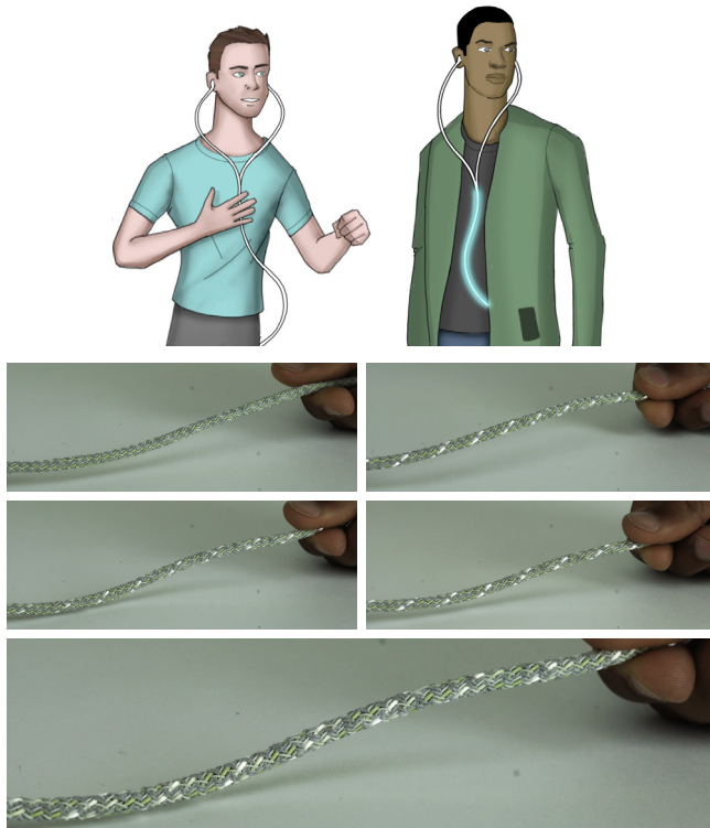
Figure 9. I/O Braid’s capability to sense touch and rotation input along the length of a headphone cord allows less precise input when on the go, for example, when jogging. The integrated visual feedback can be used to communicate phone connection or music status. This functionality could help signal social cues such as interruptibility, to onlookers. The photos show how flowing light can be used for directional feedback.
