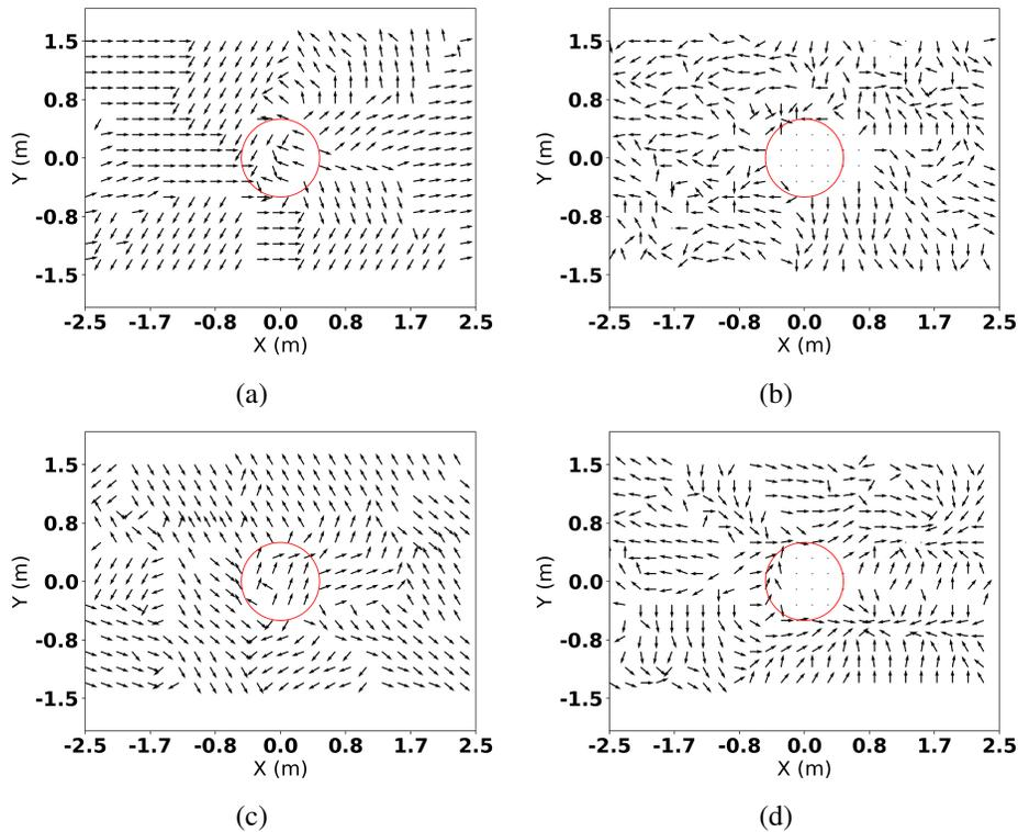
Fig. 7. RL actions as a function of position given by the actor net (a, c) and critic net ((b, d), actions that lead to the highest state-action value). The top and bottom rows show the obstacle (red circle) with deterministic and stochastic motion, respectively.
