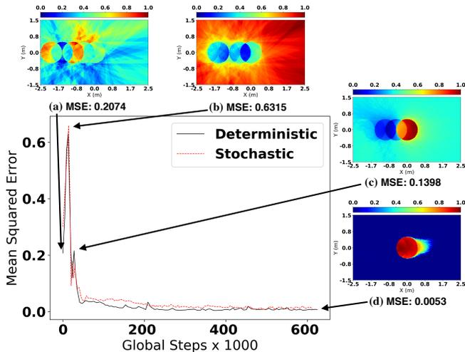
Fig. 4. MSE between  $V_{SR}$  and normalized  $V_{RL}$  as a function of global step (main figure) for deterministic (solid black) and stochastic (dotted red) obstacle motions. RL collision probabilities are shown at initial state (a), the first peak (b), the second peak (c) and convergence.
