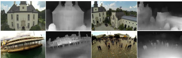
Figure 7. Frames from from YouTube and learned disparity maps. The camera intrinsics are learned.
