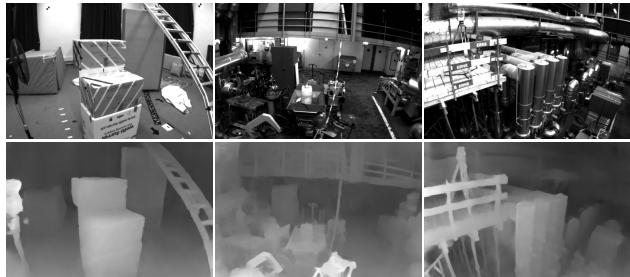
Figure 8. Frames from EuRoC [5] and the corresponding learned disparity maps. The camera intrinsics are learned.
