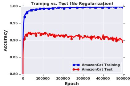
Figure 1: Training (blue) and test (red) accuracy of Alg. 1 on the AMAZONCAT-13K dataset. The non-regularized embedding-based method severely overfits to the training data.
