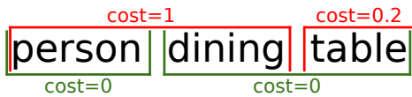
Fig. 5: Transcription segmentation. Our method assigns a cost to each subsequence of words. Then, it segments the transcription into the list of object class names that has minimal cost. In this example, segmenting into {person, dining table} has zero cost, while all other segmentations have cost > 0 , as other possible subsequences such as “person dining” are not in the vocabulary.
